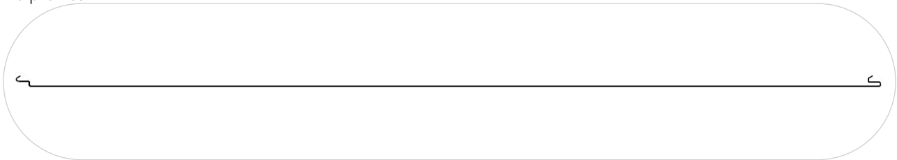
Figure 20. Geometry of wall panels with Secret Fix locking system (PWT SF)
