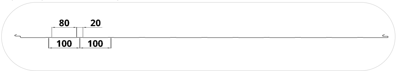
Figure 19. Types of profiles on the internal face of PWT Z panels
